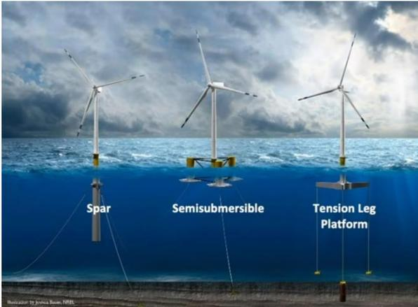
Floating wind technology accesses deepwater sites, like those off the West Coast, where the power potential runs deepest. Floating wind offers significant advantages in higher yield/capacity factors, ease of installation and minimal visual impact.
