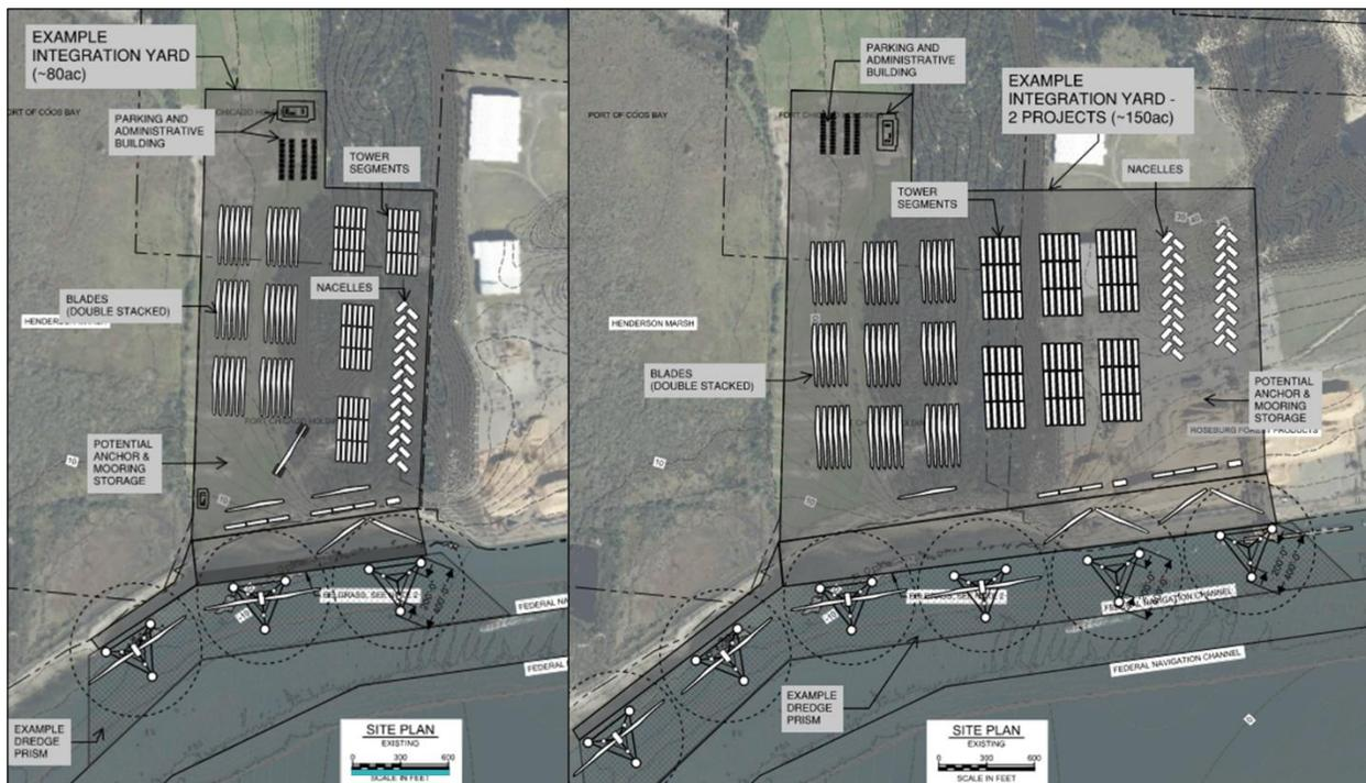
**Figure 13. Schematic-level integration site concepts to support one FOW project at a time (Example Development Scenario A, left panel) and two FOW projects at a time (Example Development Scenario C, right panel).**
