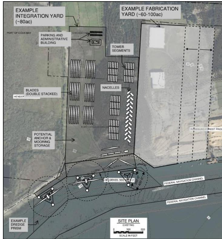
Figure 15. Schematic showing example footprint of integration & fabrication facilities.
