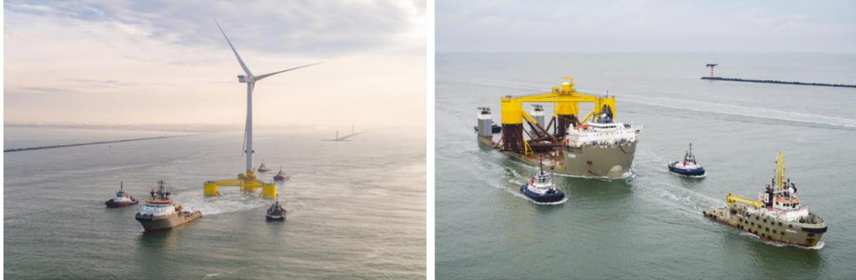
**Figure 10. Example of wet-tow of an integrated unit (left) and dry-tow of a floating foundation (right). Source: Boskalis.**
