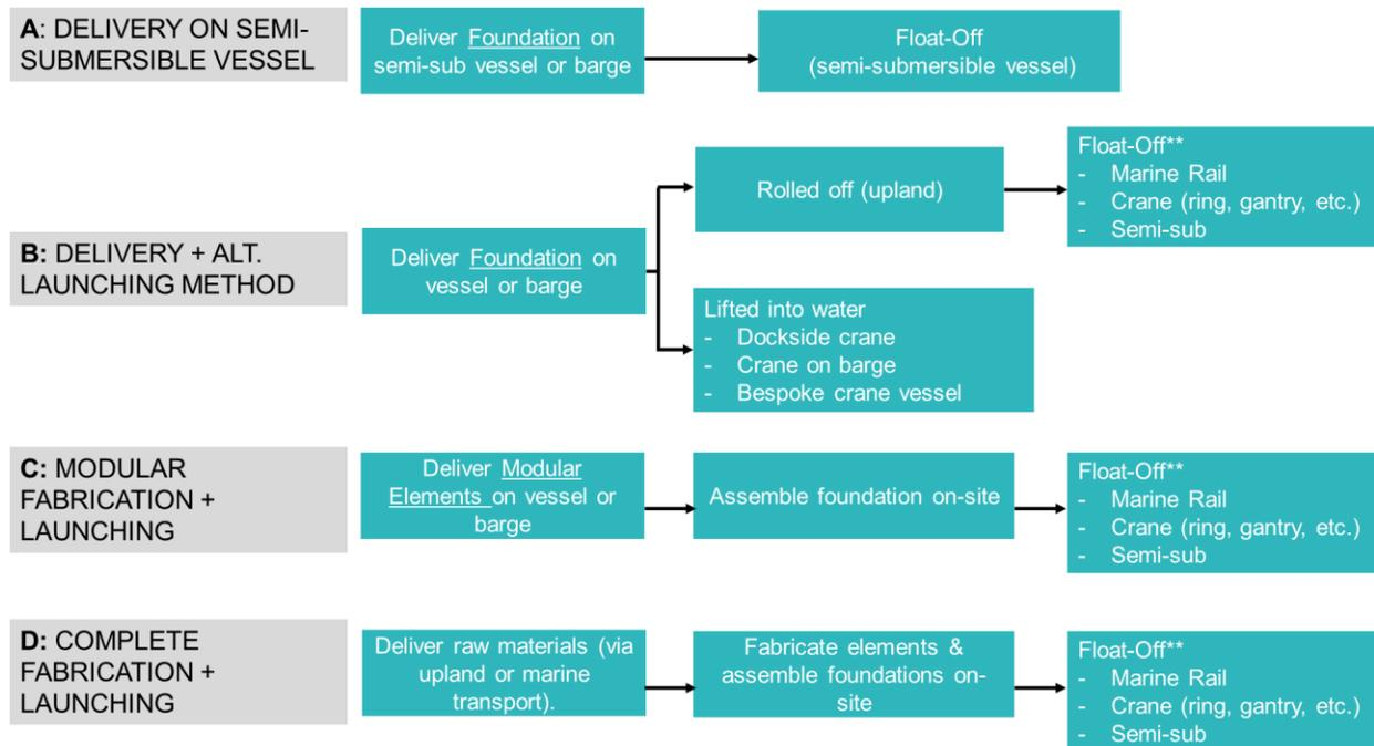
Figure 16. Foundation delivery/assembly options in Coos Bay.
