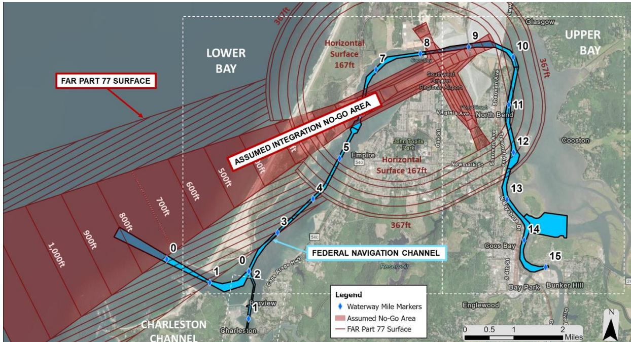
**Figure 7. Assumed WTG Integration No-Go Area (red shaded area) based on FAR Part 77 airspace surface. FAR Part 77 surface elevations shown in feet relative to mean sea level.**
